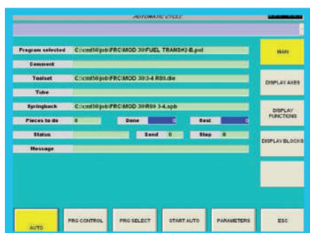
Automatic menu: Produces part in automatic mode by selecting a program from a list with graphic representation of part.
