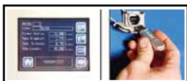
INTERACTIVE TOUCHSCREEN WITH USB PORT FOR PROGRAM STORAGE
